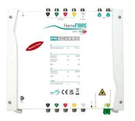
Optical transmitter that can distribute up to 4 satellites on a single fiber using CWDM (Coarse Wavelenght Division Multiplexing) technology. Innovative solution that allows the transmission of the entire TV band, FM, and an orbital position on a single fiber. Output power 7 dBm SAT + TV + FM, wavelength 1310 nm. (dimensions 230x230x50mm). The transmitter can be installed near the dish in a waterproof box thanks to the separate power supply.
